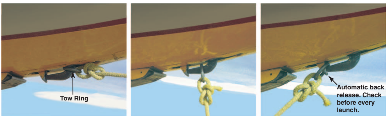
Figure 7-13. Testing the towhook.
